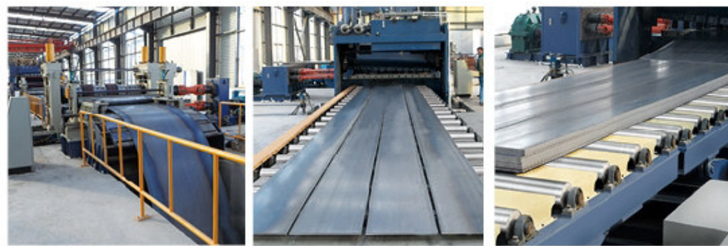
4~16×2200 Leveling and cutting line
