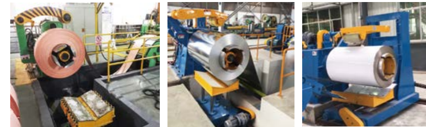
▶ 悬臂式无支撑 Cantilever only (no OBBS) L \leq 10\text{T}
