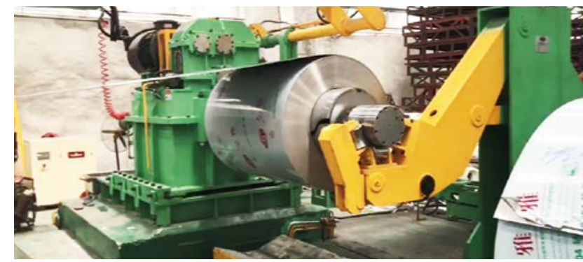
▶ 油磨线开卷 Uncoiler for No.4/HL line L \leq 25\text{T}
