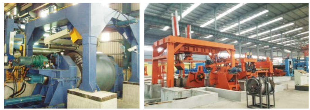
▶ 双头式龙门压料 Double head type gantry hold down arm H \leq 40\text{T}
